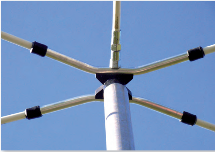
Fig. 2: The 'spider' in the centre of the antenna is of simple design. The vertical running pole (vertical in the picture but horizontal in Fig. 1) goes out to become the support point for the common feed-point, as shown in Fig. 3.
